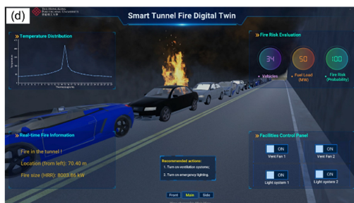
Fig. 3. Smart Tunnel Fire Digital Twin System
