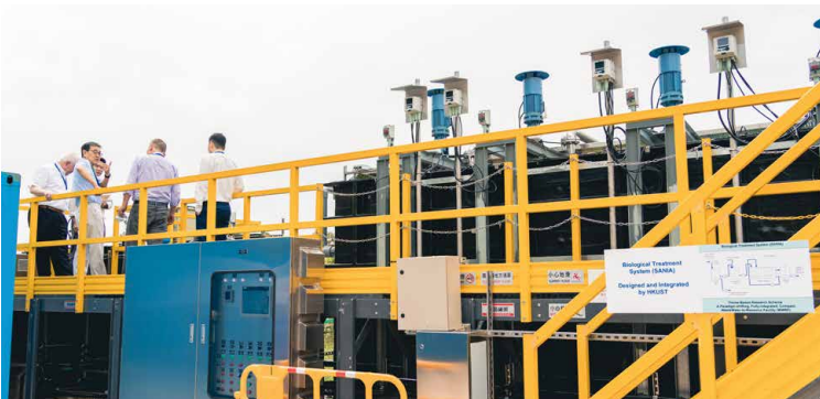
Pilot-scale testing of a novel wastewater technology—SANIA SANIA 創新工藝技術的中試研究
